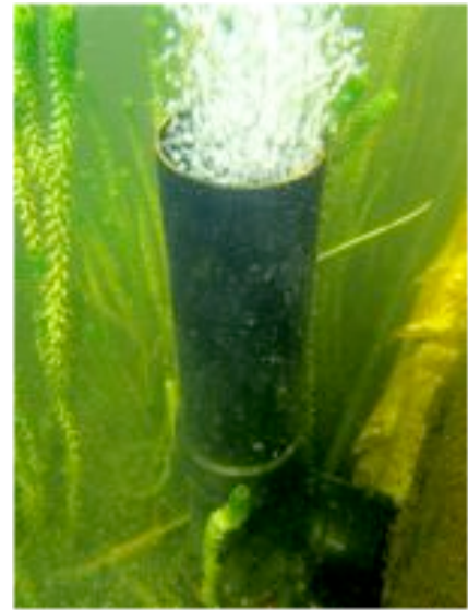
This Bubble Pump consists of a couple of lengths of 110mm dia. standard drainage pipe and a 90 degree bend fitting.
