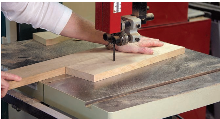
Cut the curve. I traced my pattern onto each foot and made the cuts at the band saw.
