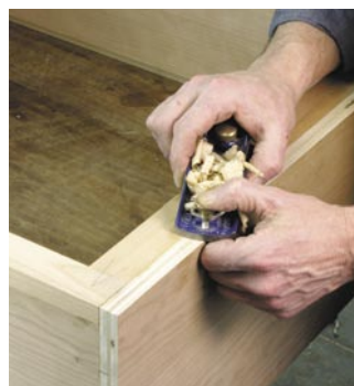
It's safer to trim the solid wood parts down to the plywood parts. The block plane works quickly against an edge or against the veneer.
