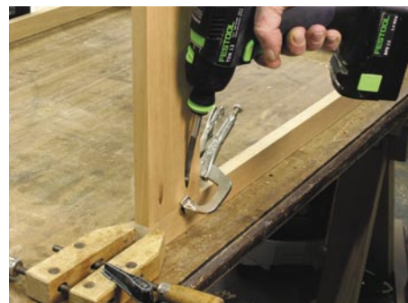
The face frame is put together with pocket screws before being glued in place on the assembled cabinet box. Two clamps hold the stile on edge so that I can see and reach both sides of the joint.
